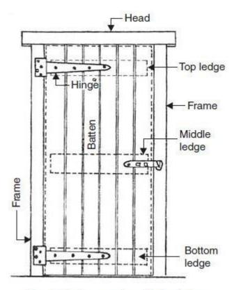
Fig. 8.21. Battened and ledged door
