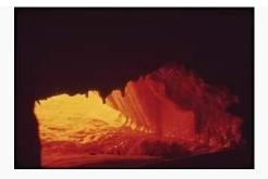
The hot end of a glassworks is where the molten glass is formed into glass products, beginning when the batch is fed into the furnace at a slow, controlled rate by the batch processing system (batch house). The furnaces are natural gas- or fuel oil-fired, and operate at temperatures up to 1,575°C. The temperature is limited only by the quality of the furnace's superstructure material and by the glass composition. Types of furnaces used in container
