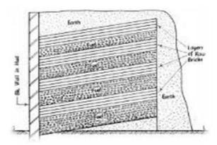
After these alternate layers of the bricks and fuel the top surface is covered with the mud so as to preserve the heat. Fire is ignited at the bottom, once fire is started it is kept under fire by itself for one or two months and same time period is needed for the cooling of the bricks.
