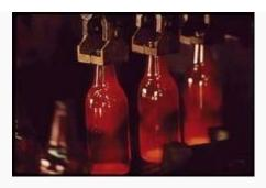
There are, currently, two primary methods of making a glass container: the blow and blow method, used for narrow-neck containers only, and the press and blow method used for jars and tapered narrow-neck containers.
