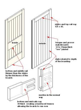
This type consists of a solid timber frame, filled on one face, face with Tongue and Grooved boards. Quite often used externally with the boards on the weather face.
