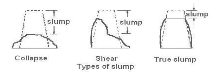
This test is usually used in laboratory and determines the workability of fresh concrete when size is about 40 mm maximum. The test is carried out as per specification of IS: 1199-1959.
