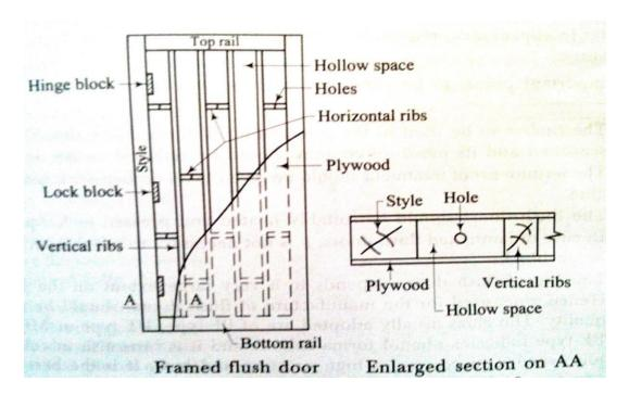
It consists of styles, rails, horizontal ribs, vertical ribs, and plywood. As shown in fig.
