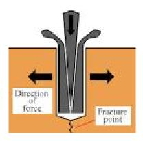
The wedging is adopted for costly stratified rocks which are comparatively soft such as laterite, marble, limestone, sandstone, etc. The wedging is preferred to the blasting, wherever possible.
