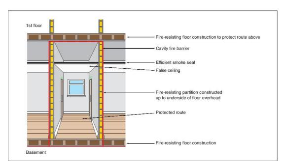
Figure 1: Fire-resisting construction
